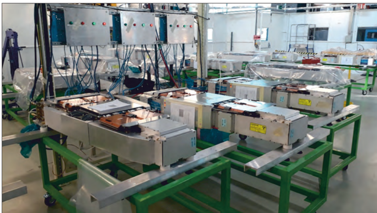
Fig. 1. Stand for long-term testing of the performance of ME1/1 detectors
