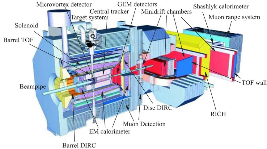
Fig. 3. 3D view of the PANDA spectrometer
