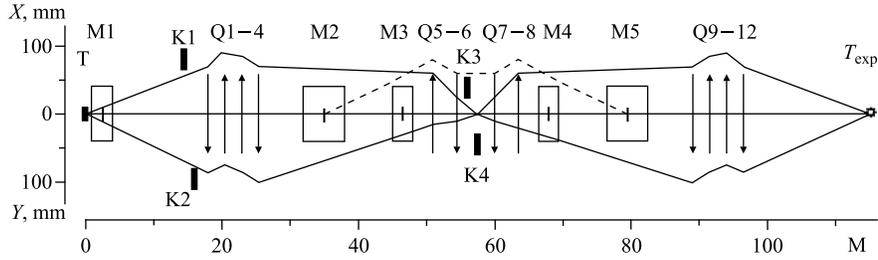
Fig. 9. Optical scheme of the polarized particle channel
