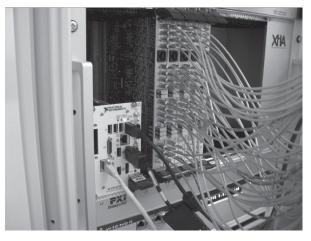
Fig. 3. PXI chassis with XIA digitizers and a NI controller
