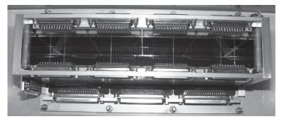
Fig. 1. Si strip detector of the well type
