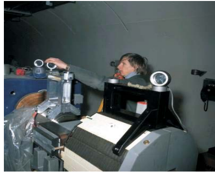
Fig. XII. Socket for laboratory metrology and specific gauge (CERN TS-SU-EM library)
