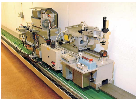
Fig. XIV. Measure chariot of the calibration bench at CERN (CERN TS-SU library) and result of an electro-optic distance-meter calibration
