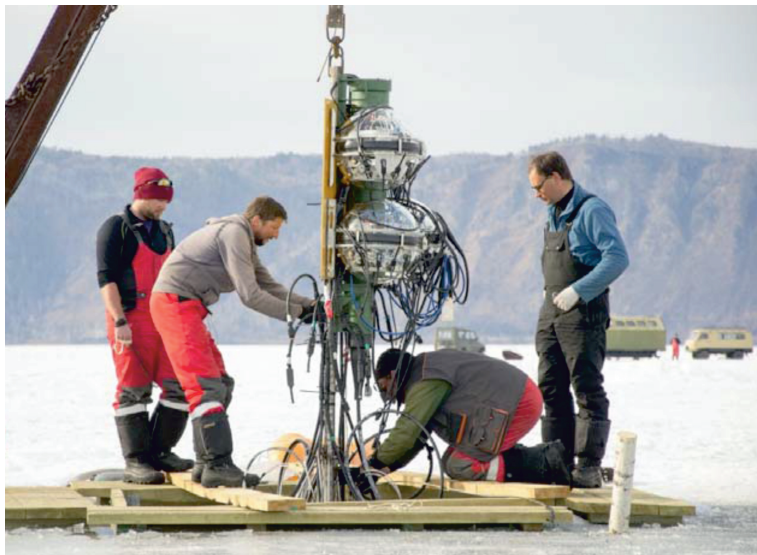
The assembling of the optical modules garland before dipping it into the Baikal
