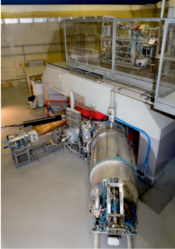
The DC-280 cyclotron — the basic facility of the SHE Factory
