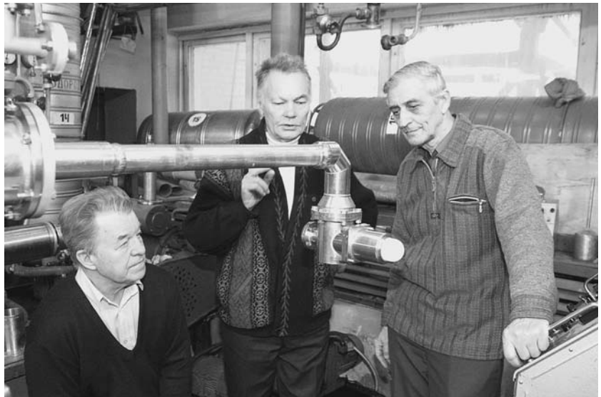
Veksler and Baldin Laboratory of High Energies. Liquid hydrogen target for the project «Thermalization» manufactured in the Cryogenic Department of VBLHE. From left to right: Yu. Borzunov, V. Nikitin, L. Golovanov
