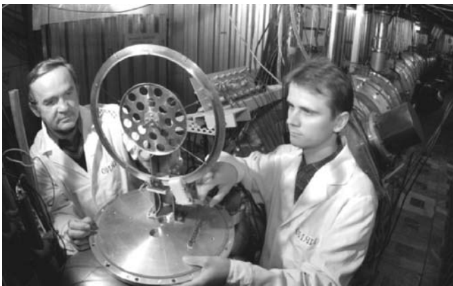
Veksler and Baldin Laboratory of High Energies. General view of the station mechanism of the Nuclotron internal target before assembling it into the accelerator vacuum chamber
