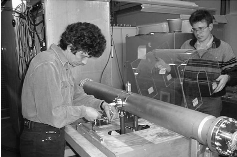
Laboratory of Particle Physics. Stand-by tests of the damping system for transverse oscillations of a particle beam at CERN's LHC
